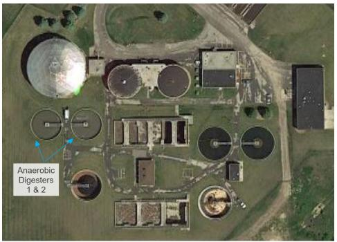
Figure 1 | Aerial View of the Plymouth Utilities' Wastewater Treatment Plant
